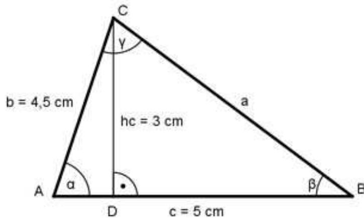
$$\sin \alpha = \frac{h_c}{b} = \frac{3 \text{ cm}}{4,5 \text{ cm}} = 0,6667 \rightarrow \alpha = 41,8^\circ$$
